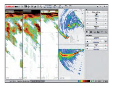
Up to five inspection beams (three shown here) can be trained and tilted individually while maintaining the overview with the horizontal fan and vertical slice.
