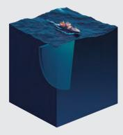
The SN90 has one vertical slice that can be trained in any direction within the fan. This will give full control of the edges of the school during setting of the net.
