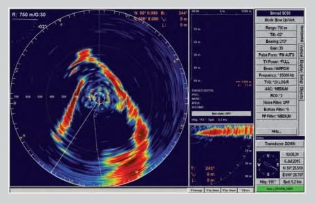
The completely noise free capability of the SC90 makes it easy to see wanted targets and avoid spending time interpreting the sonar picture. Even in shallow water, the picture is clean and easy to understand.
