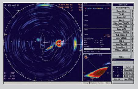
In short range, which is the reason to have a second sonar, the sharp well defined echoes due to the very high resolution are important. Like in the case to the left, it is very useful to have a well defined "backside" of the school, especially for purse seiners, in order to get a general feeling of the size of the school before setting the net.
