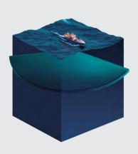
The SN90 has a 160° fan that is tiltable from 0° down to 90°. This will enable to see the purse seine during the whole setting of the net.
