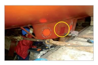
Installed looking to the port side of the vessel together with horizontal looking ES70 echosounders previously installed.
