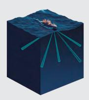
The SN90 has five individually steerable inspection beams that can be trained and tilted with any frequency between 70 and 110 kHz. The inspection beam will give a detailed high resolution echogram.
